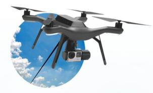
Communication also takes place through the cable, **preventing jamming and interception.** The safety ensured by tethering the UAV to ground via a cable makes it easier to gain permission from civil aviation authorities for use in civil and controlled airspace.
